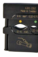
OSW0360 Crimping die for Elpress MOBILE tool for crimping through connectors with heat shrink insulation 0.3-0.75 mm 2 and 4-6 mm 2 . AWG 11-9.
